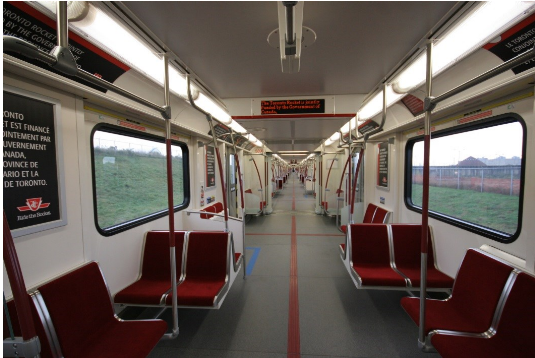
Figure 3: Open-gangway Toronto Rocket train
